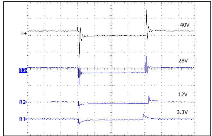
Figure 14: Output voltage response for 28V input; 3.3V, 12V, 28V, 40V output to step change in load current (50%-75%-50% of Iout max; di/dt=0.1A/uS). Load cap: 100uF electrolytic cap, Vout (500mV/div); (5mS/div)
